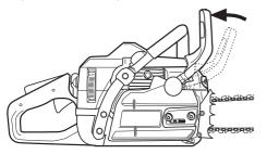
Remove the bar nuts and remove the clutch cover (chain brake). Take off the transportation ring (A).
